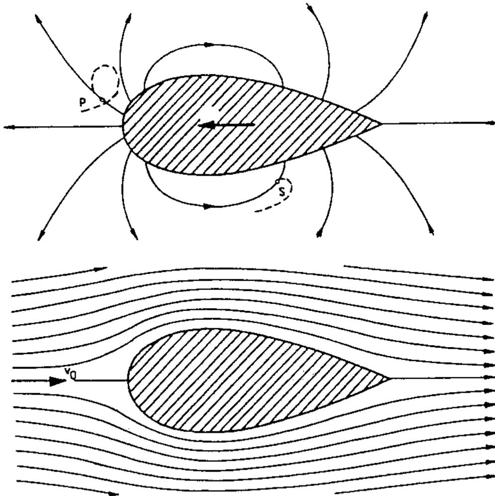
Figure 8 : Streamline patterns of flow around body, (5).
