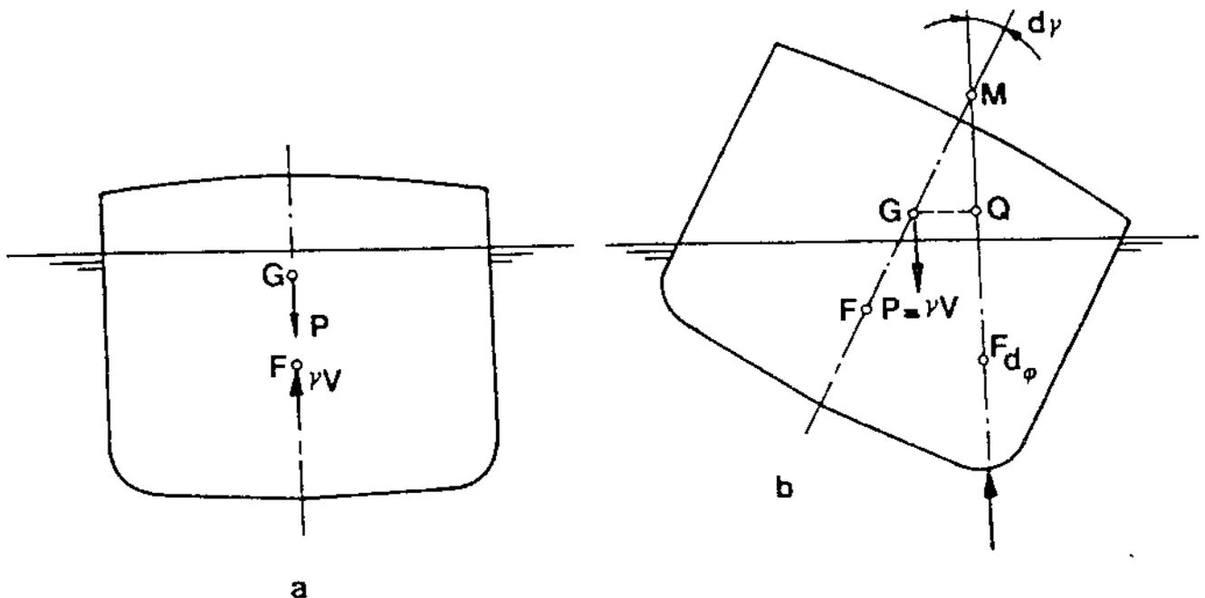
Figure 5: Partly submerged body in two positions (6).
