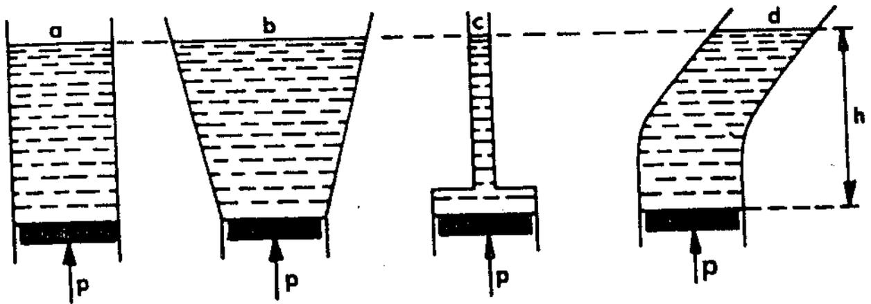
Figure 3a : Pressure on the bottom of a vessel, (6)
