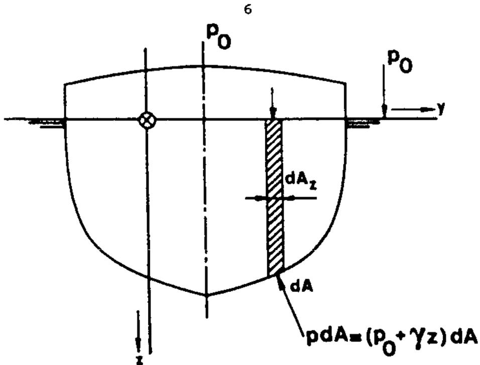
Figure 3b: Pressure on the hull of a body (6).
