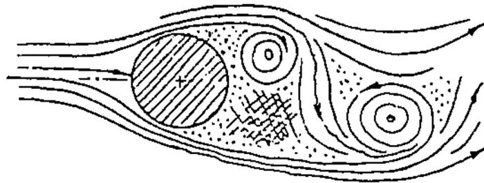
(C) CYLINDER BETWEEN  $R_d = 10^4$  and  $10^5$ ; VORTEX STREET WITH  $C_D = 1.2$ .
