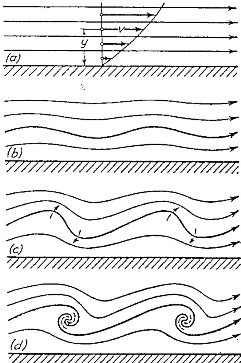
Figure 11 : Growth of a disturbance in a flow, (5).
