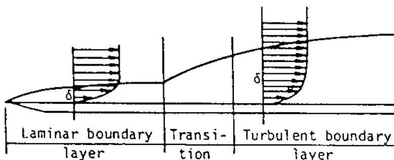
Figure 13 : Boundary layers along flat plate, (7).
