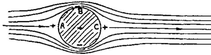
(A) FLOW PATTERN OF CIRCULAR CYLINDER IN NON-VISCIOUS FLOW; NO DRAG.
