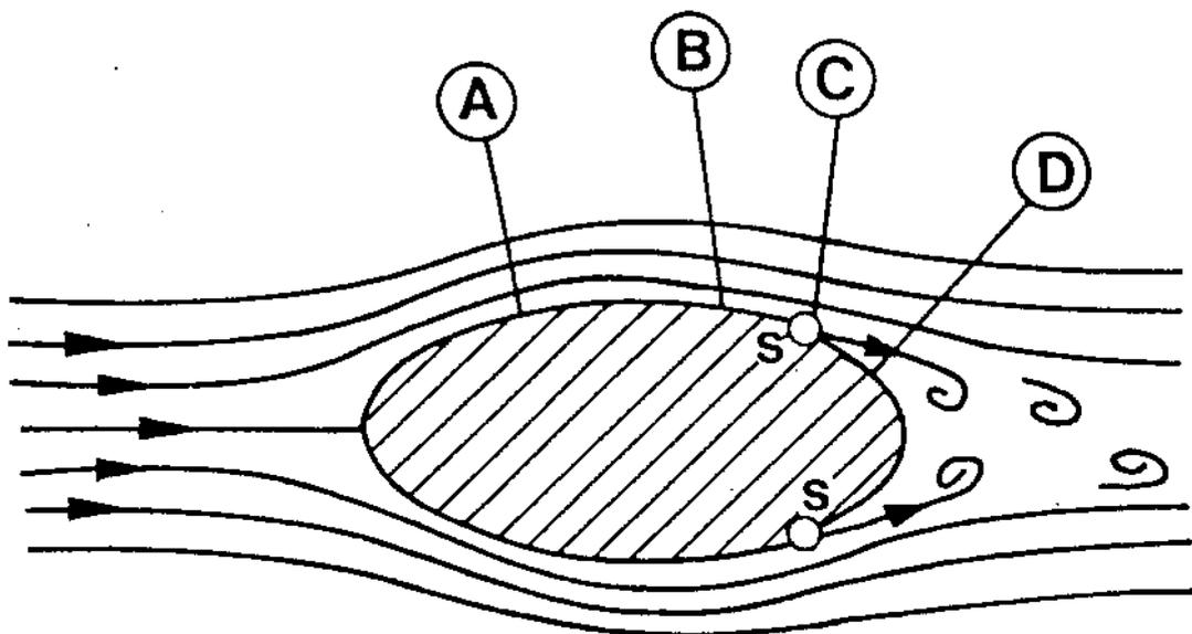
Figure 15 : Separation of flow at aft end of body, (3).
