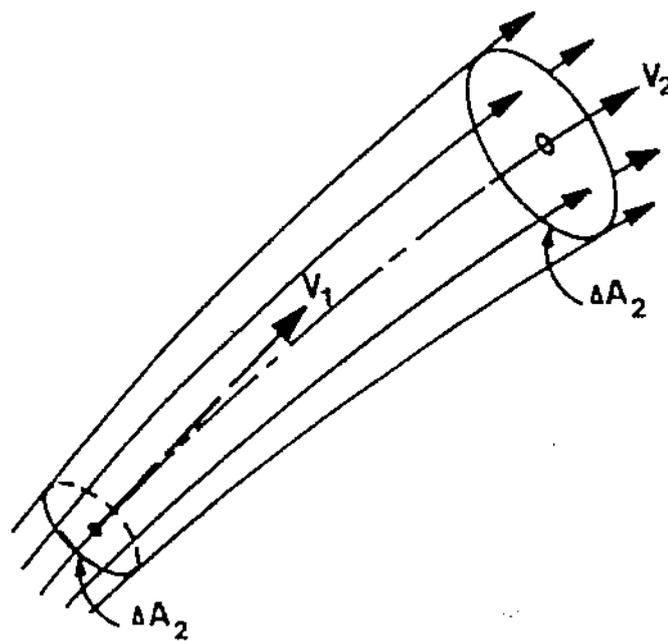
Figure 7 : Streamlines and velocity vectors (top); elementary streamtube (bottom), (5).
