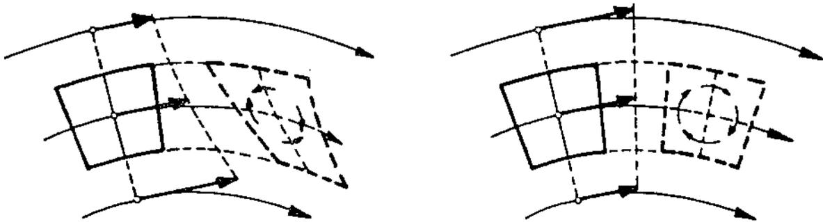
Figure 9 : Types of motion of fluid elements, (5).
