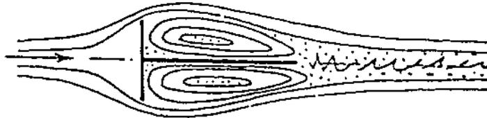
(D) PLATE WITH "SPLITTER" DEVICE IN WAKE;  $C_D = 1.5$ .
