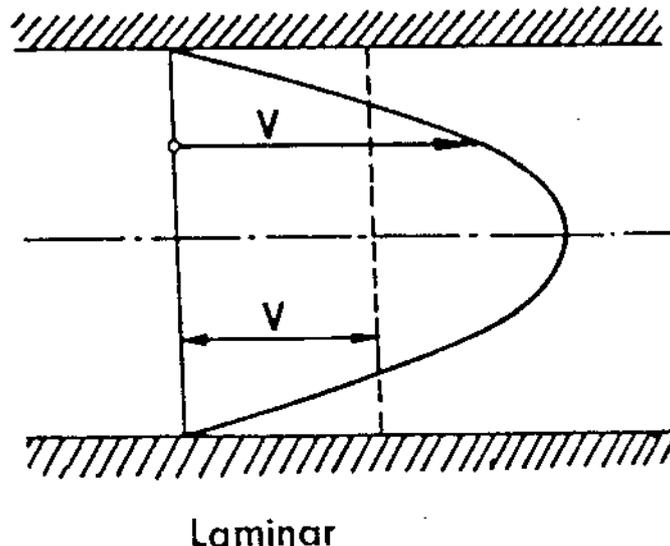
Figure 12a : Laminar flow in a duct, (5).
